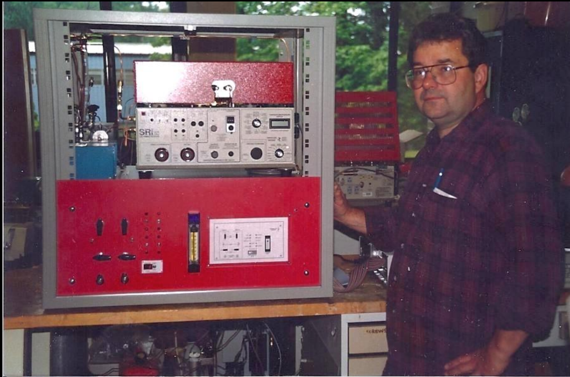
The pCO 2 gas chromatograph system Tom packaged for Taro's ocean program
