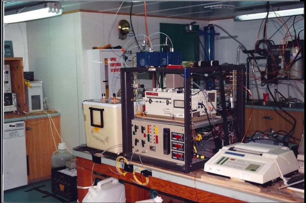
pCO 2 GC and IR Systems aboard the RV/IB N B Palmer
