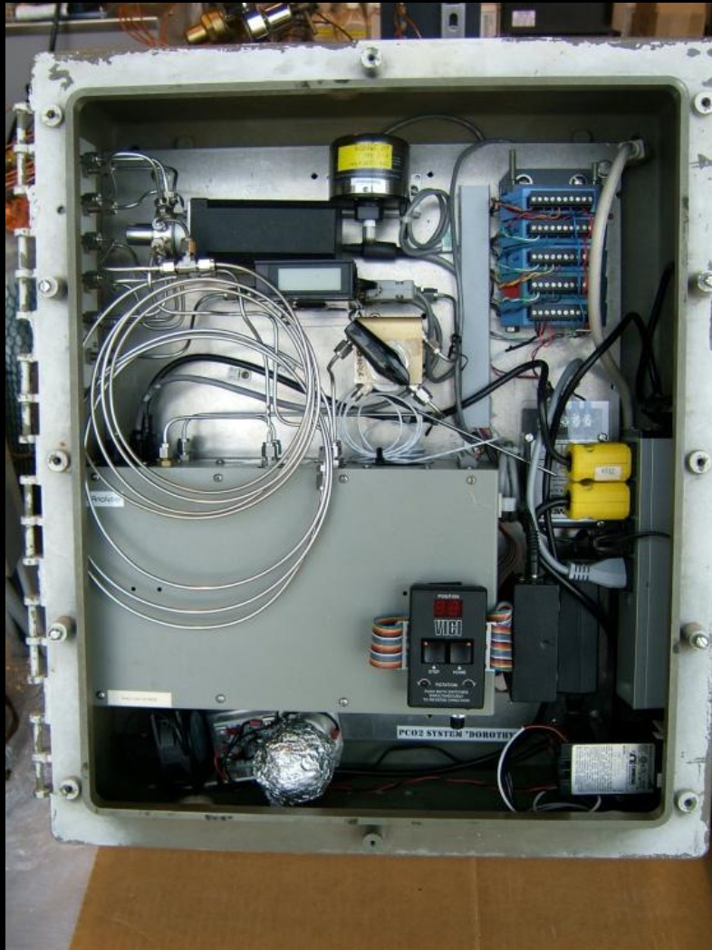
Real-time pCO 2 IR Analyzer
