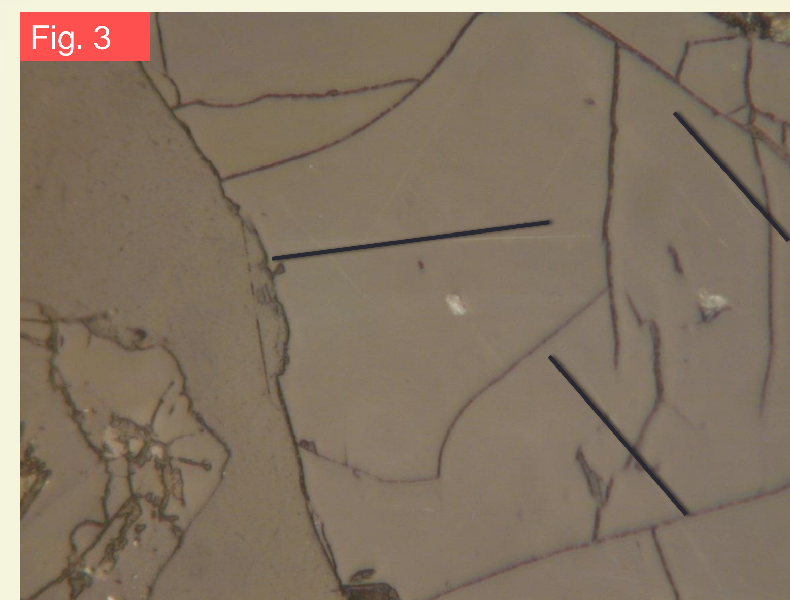
Fig. 3: Photograph of a shocked quartz grain from ELT 32-43. The straight black lines represent the three different sets of lamellae in different orientation.
