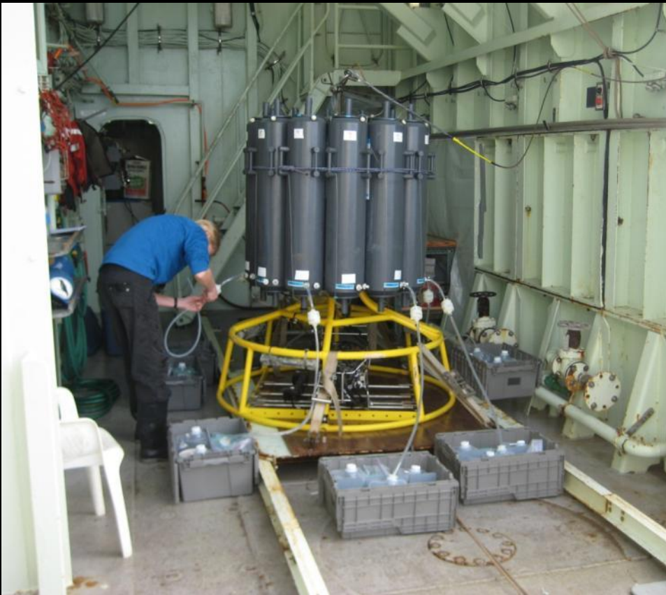
Katharina Pahnke using the pressurized rosette for large volume sea water samples
