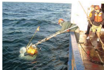
Crew members on the SUNY Stony Brook research vessel Seawolf retrieve an ocean-bottom seismometer during a test deployment off the coast of New Jersey. Credit: Ken Kostel
