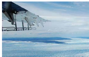
Magnetometers and gravimeters—instruments more commonly used to study the seafloor from ships—together with ice-penetrating radar and laser altimeters are being used by Michael Studinger and Robin Bell to peer beneath miles of ice from an airplane (shown above Greenland). Credit: Michael Studinger
