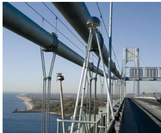
GPS antenna installed by Mikhail Kogan and his colleagues on the Verrazano-Narrows Bridge to study the motions imparted on the bridge by more than 37,000 runners in the New York City Marathon. Credit: Mikhail Kogan
