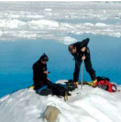
[above] Leigh Stearns from the University of Maine and Andreas Ahlström from the Geological Survey of Denmark and Greenland install a GPS station on Helheim Glacier in East Greenland as part of Meredith Nettles’ recent work to monitor glacial earthquakes. Credit: Gordon S. Hamilton
