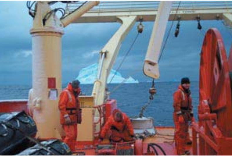
1. Deployment of a mooring in the northwest Weddell Sea. Division scientist Gerd Krahnmann is seen here attaching an instrument onto the mooring cable that will allow researchers to take temperature and conductivity measurements, which are then used to calculate water salinity and pressure. Credit: Phil Mele
