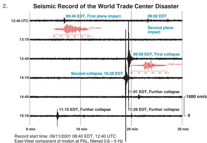
2. Two hours of seismographic information recorded by the Lamont Cooperative Seismic Network on the morning of Sept. 11, 2001 show the airplane impacts and the subsequent collapse of the World Trade Center's two towers.
