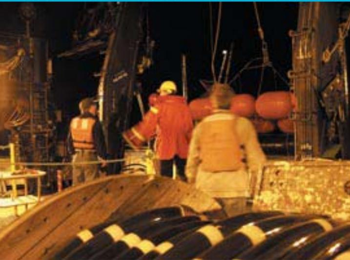
1. Technicians and crew of the Juan de Fuca MCS survey, during night operations, launch a hydrophone array's tail buoy, which communicates its position 6.2 km behind the R/V *Ewing*.
