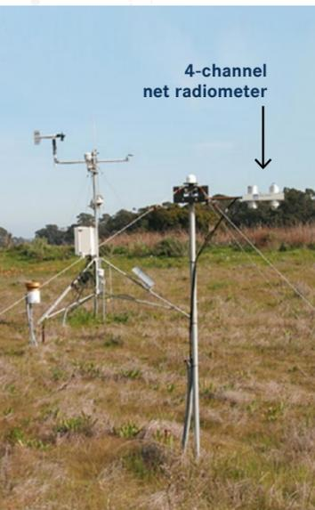
4-channel net radiometer
